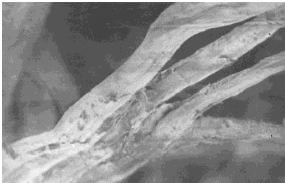
Figure 10 SEM micrograph of treated (consolidated) jute fiber.
